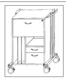
Filing drawer DIN A4, shelf, below inset for X-ray folders with vertical subdivision. Partition wall for shelf, below small shelf and two small drawers 100 and 200 mm high, 1 push handle.
