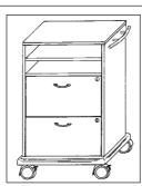
2 shelves, 2 filing drawers DINA 4, with integrated weight against inclination of the trolley, when the drawers are pulled out.
