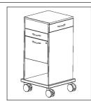
Basic trolley of special size with side push handle, pull-out laptop computer drawer at the side, holder for Kensington lock, 1 drawer, 10 cm high, 1 DIN A4 filing drawer. Castors Ø 100 mm, 2 are lockable.
