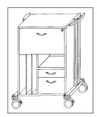
Filing cabinet DIN A4, shelf, below inset for X-ray folders with vertical subdivision. Partition wall for shelf, below small shelf and two small drawers 100 and 200 mm high, 1 push handle.
