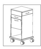
Basic trolley of special size with side push handle, pull-out laptop computer drawer at the side, holder for Kensington lock, 1 drawer, 10 cm high, 1 DIN A4 filing cabinet. Castors Ø 100 mm, 2 are lockable.
