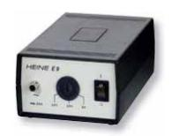
2.5 V/3.5 V/6 V/0.8 A max. (Suitable for all cord handles with Cinch plug.) For all 2.5 V and 3.5 V instruments and for the 6 V lamp handle. Dimensions: Width 110 mm, Height 70 mm, Depth 170 mm. Weight: 660 g.
