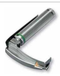
The FlexTip+ is a Macintosh laryngoscope blade with a tip which is adjustable through 70°. A lever controls the tip angle during intubation to lift the epiglottis, giving a clear view of the vocal cords. Contact with the upper row of teeth and unnecessary pressure on the tongue and soft tissue are avoided.
