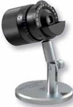
This model eye is ideal for teaching and practice. The pupil diameter and refractive error can be set exactly and are therefore reproducible. The Front holder accepts up to two trial lenses. The cyl. can be read from the graduated scale.
