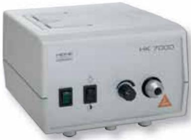
The F.O. Projector HK7000 incorporates a special long-life halogen bulb rated at 150 Watts. If more light is needed for a particular examination, a boost switch can be operated, giving up to 40% more light. Suitable for all HEINE Systems with fiber optic illumination. Dimensions: Width 177 mm, Height 125 mm, Depth 217 mm. Weight 3,700g.
