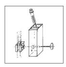
Disposable container for holding approx. 500 used needles, **made of black recycled plastic.**
